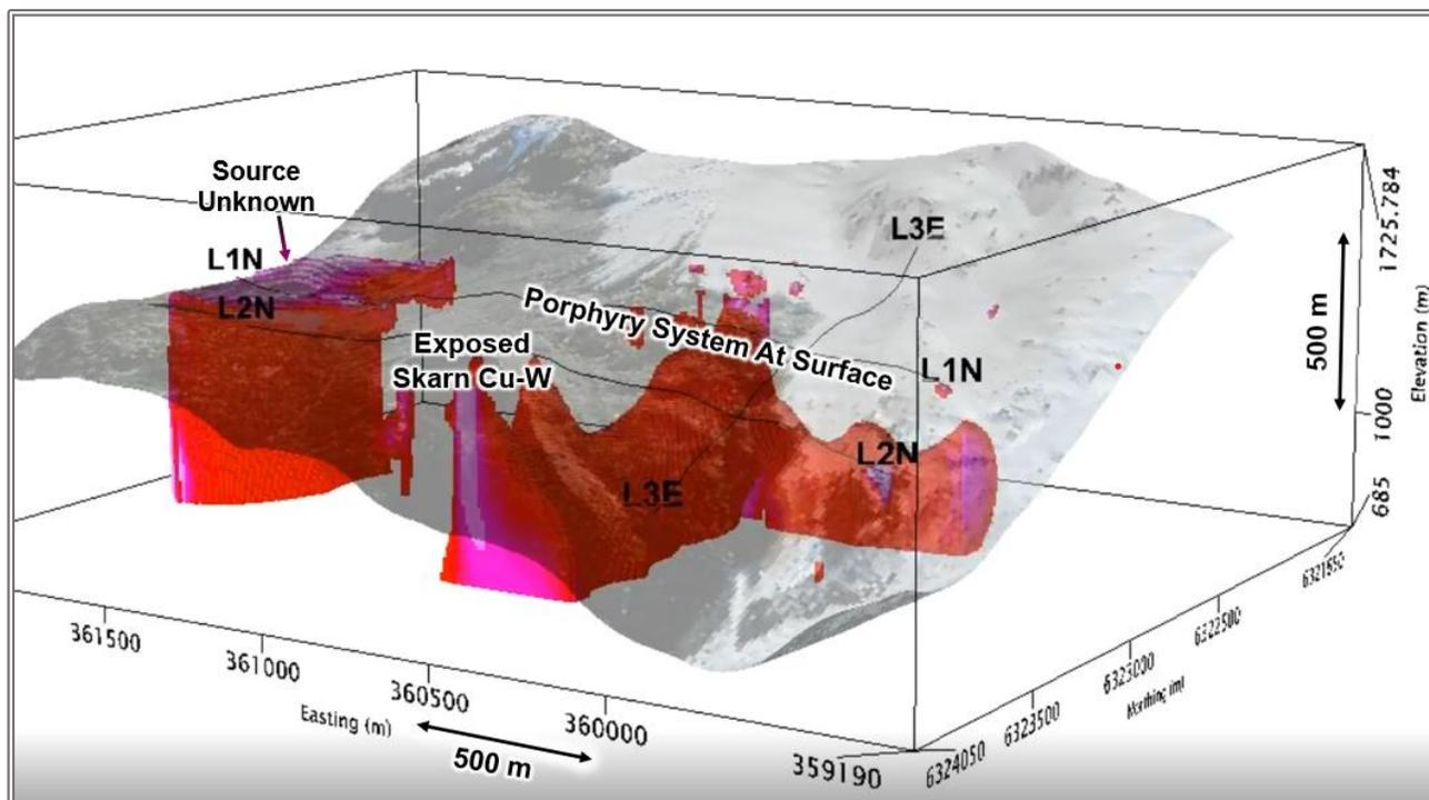
**Figure 1: Southeast looking orthogonal view of the Trek South 3D chargeability model derived from IP data. Chargeability highs in red are believed to reflect sulphide mineralization beneath the exposed porphyry and skarn mineralization.**
