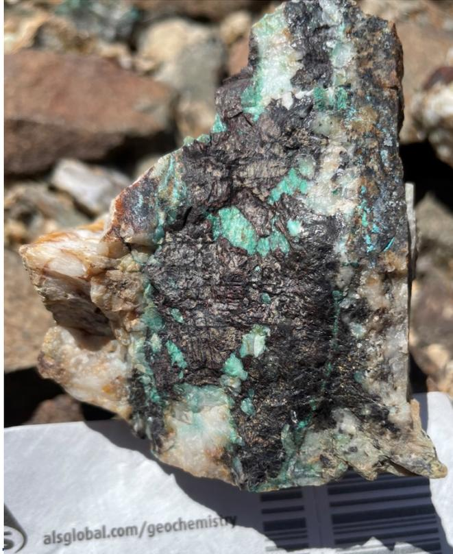
Photo #1 - Sample #E268328 from the "Au-Cu Adits" dump site. Massive, black, tarnished chalcopyrite (copper-iron sulphide) and green secondary copper mineral staining in a white quartz vein. Assayed 5.7% Cu, 1.7 g/t Au. 34 g/t Ag. One of very many such pieces at this site, some assaying up to 17.9 g/t Au.
