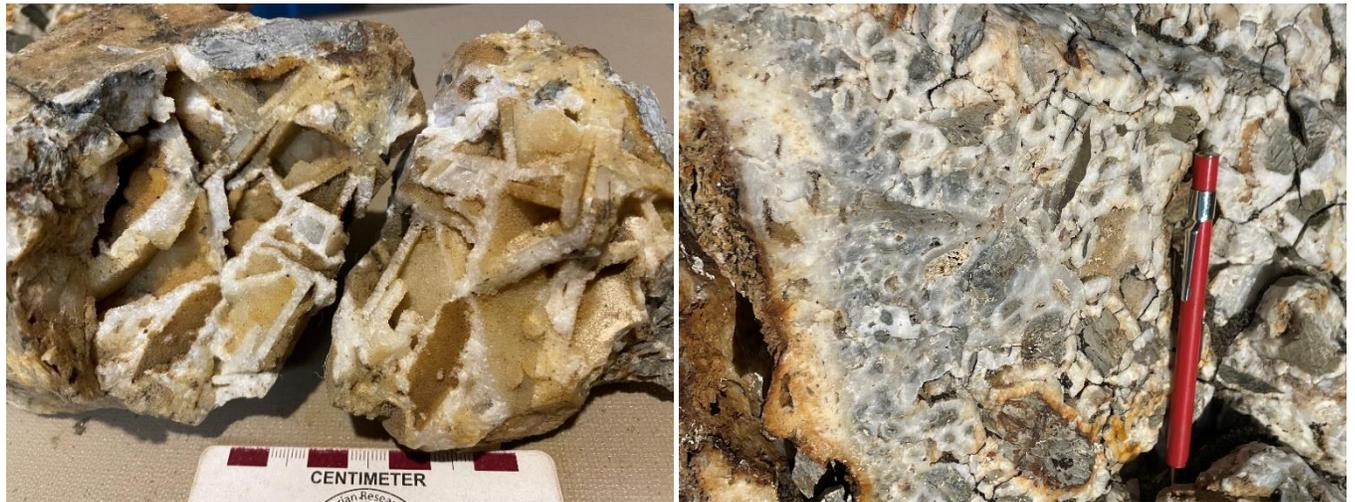
*Photo 1 (left): Spectacular quartz-lined open boxwork texture from the Angel Wing vein, indicative of the boiling zone in vein formation. Photo 2 (right): Chalcedonic and drusy quartz infilling breccia vein, Scossa 1-12 vein.*
