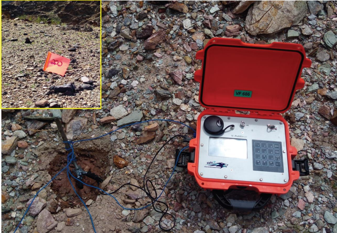
Figure 2-3: Example of Line Staking with Wireless IP Receiver (Alpha) Setup
