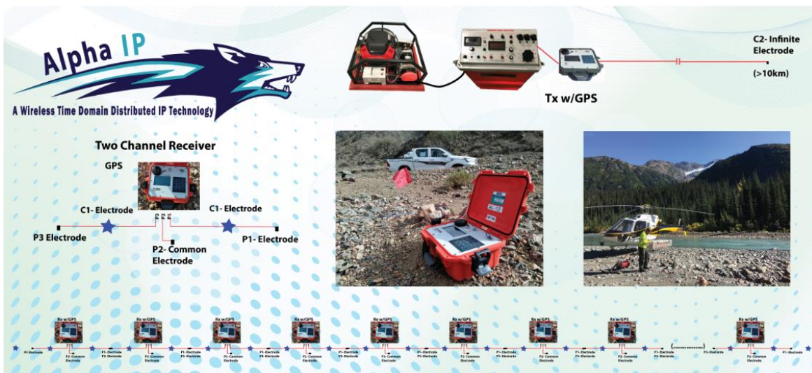
Figure 2-2: Alpha IP Schematic Spread Setup with Current Injection Offset.
