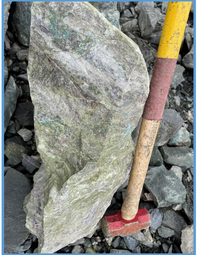
Photo 7: Epidote alteration sample with secondary copper mineral staining
