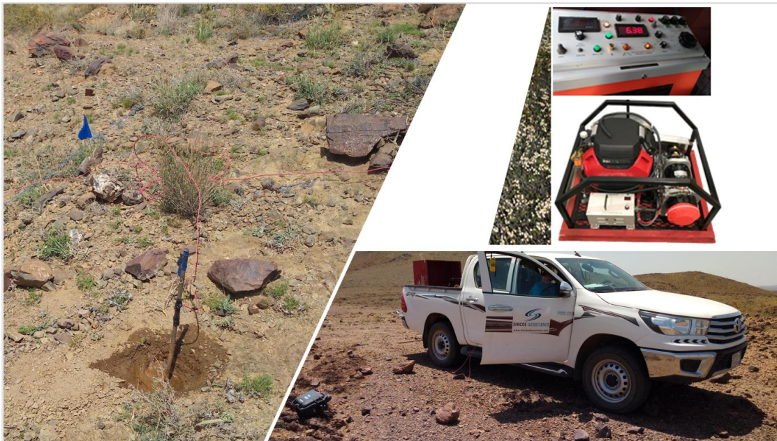
Figure 2-4: Example of Injection Dipole with Honda Motor Generator and Transmitter Setup.
